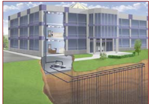
Figure 2. Schematic rendering of closed loop heat pump system. Image from www.mcquay.com
