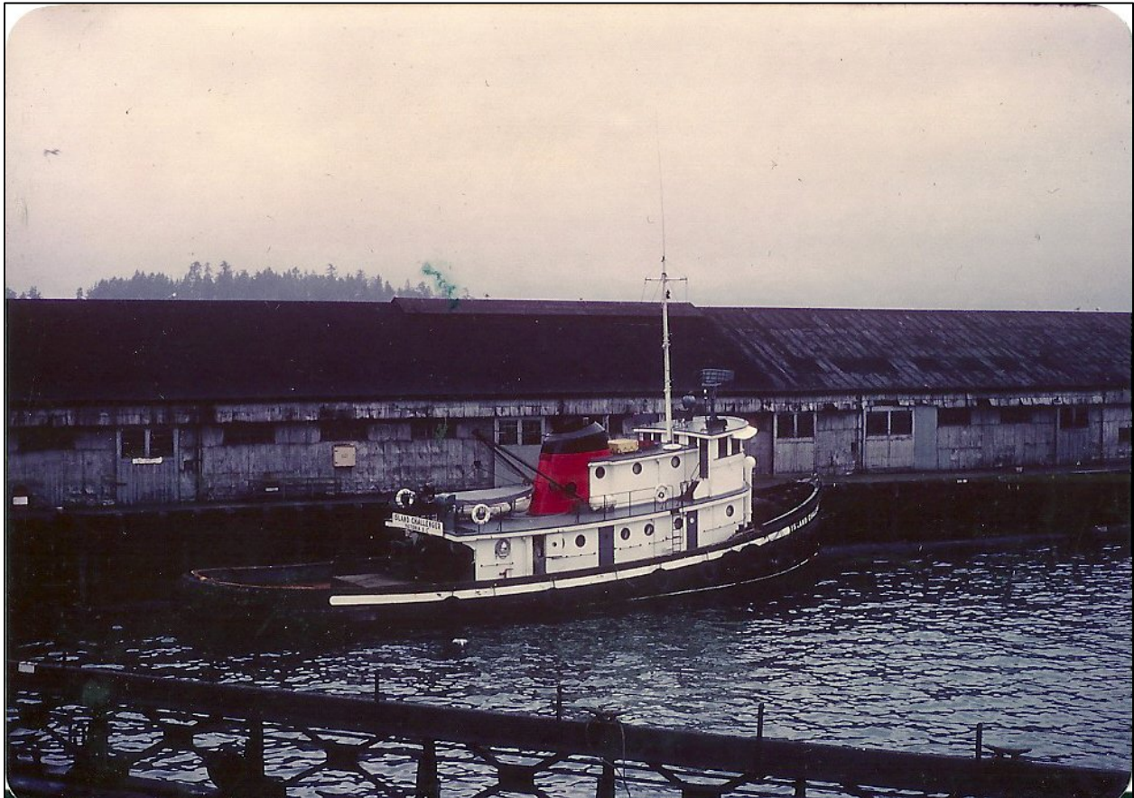
Figure 6. Island Challenger after engine replacement, note new exhaust stack and modified upper cabin (photograph – Vancouver Maritime Museum).
