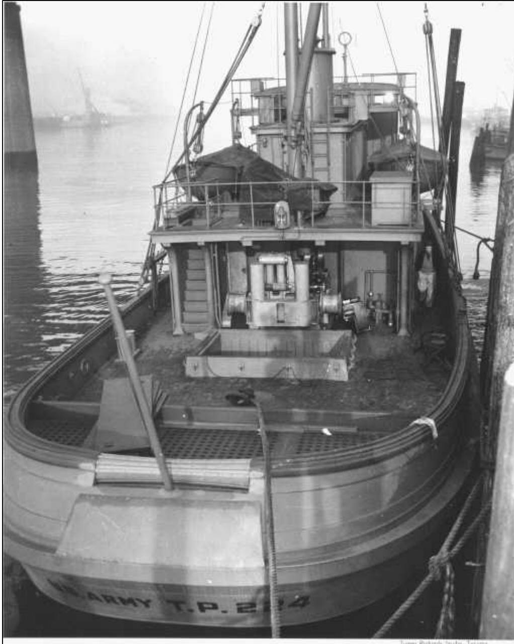
Figure 3. TP 224 at the dock, 1943. Note open working deck and tow handling equipment (photograph – Tacoma Public Library).
