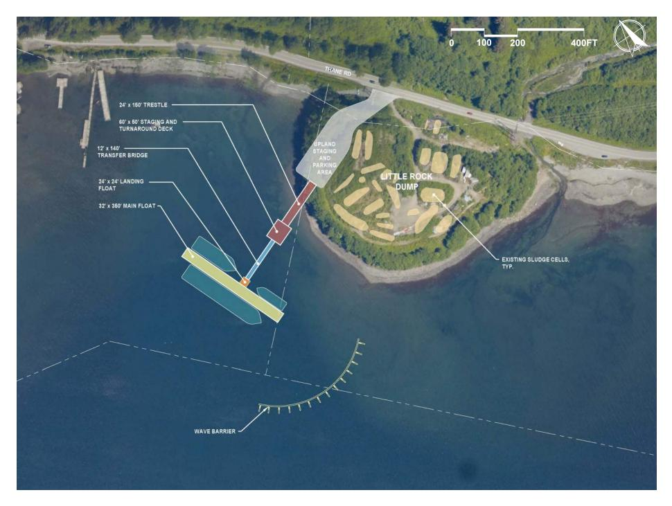
The uplands area measures roughly four acres and is currently used for storage and staging surplus construction materials by CBJ D&H. Bathymetric conditions to the north of the Little Rock Dump are favorable for siting necessary marine structures without dredging. However, wind and wave conditions along Gastineau Channel may impact moorage operations without protection.
