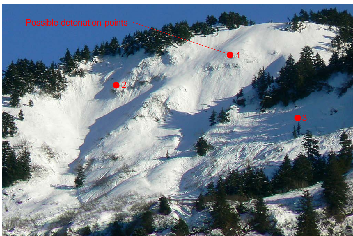
Fig. 49: Possible detonation points in the starting zone of White Subdivision avalanche path (top area above the bench).
