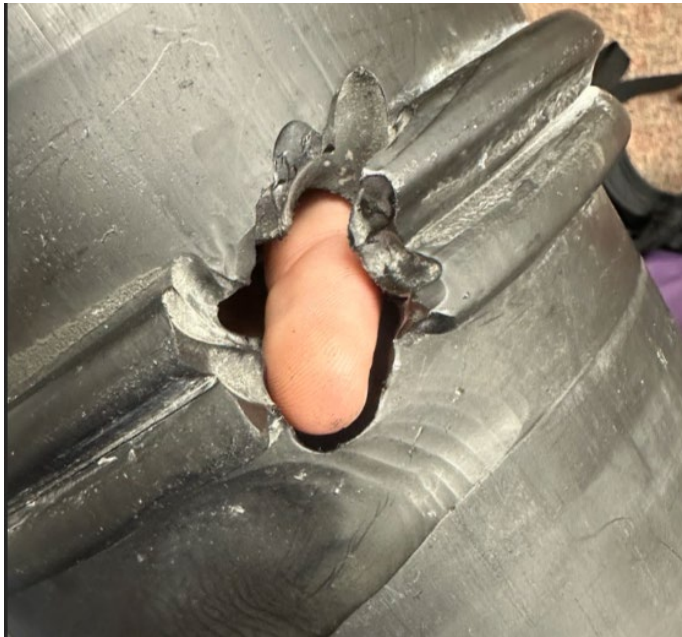
Photo 7. Inner pipe breach.
