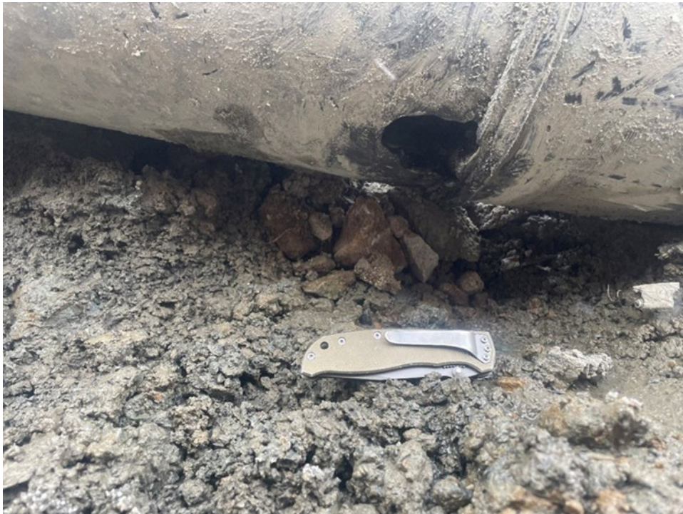
Photo 8. Outer pipe breach.
