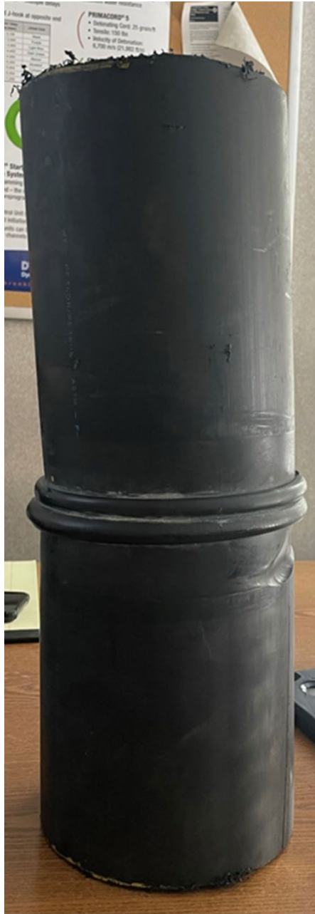
Photo 6. Misaligned Electrofusion weld at failure point.
