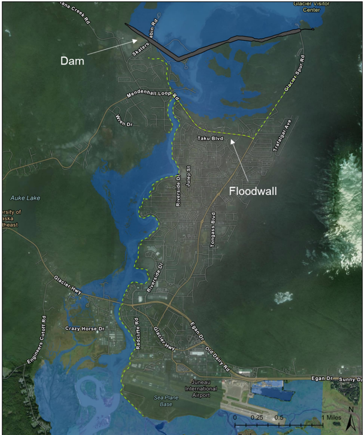
Figure 4-48 Floodwalls Shown with a Dam Release of 50,000 cfs
