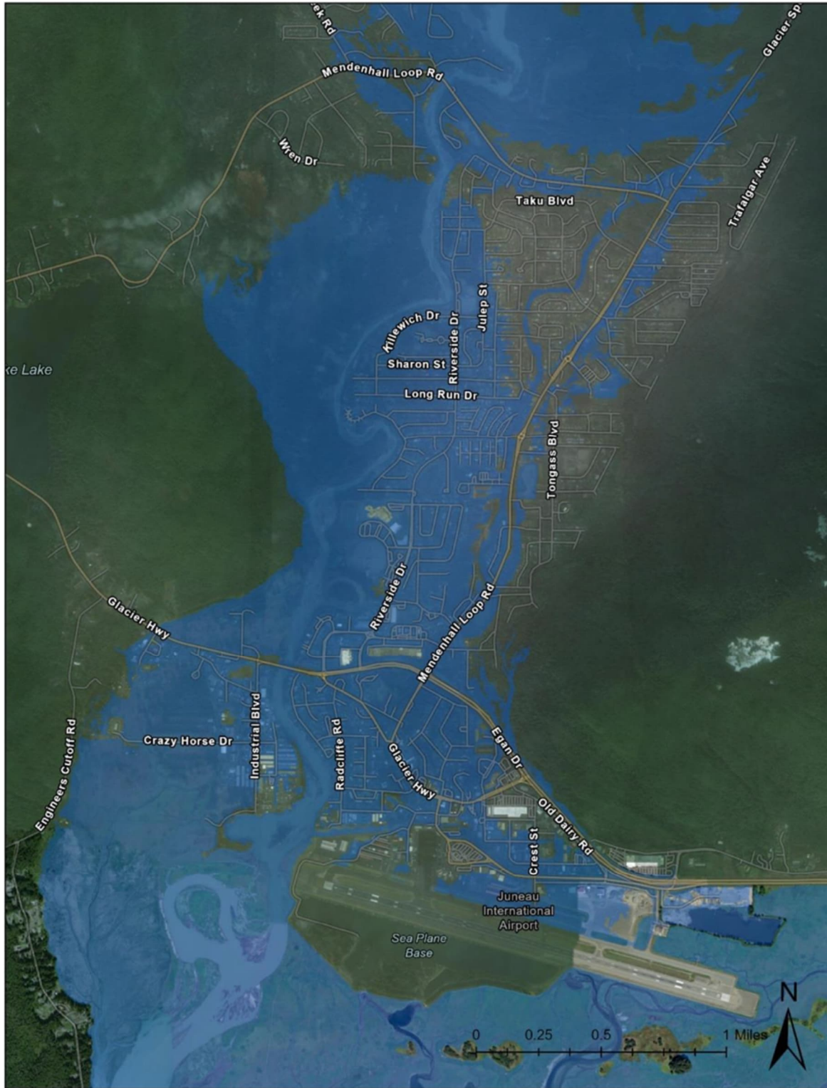
Figure 4-51 Inundation Extent with No Protection Under the Design Peak Flow of 118,000 cfs
