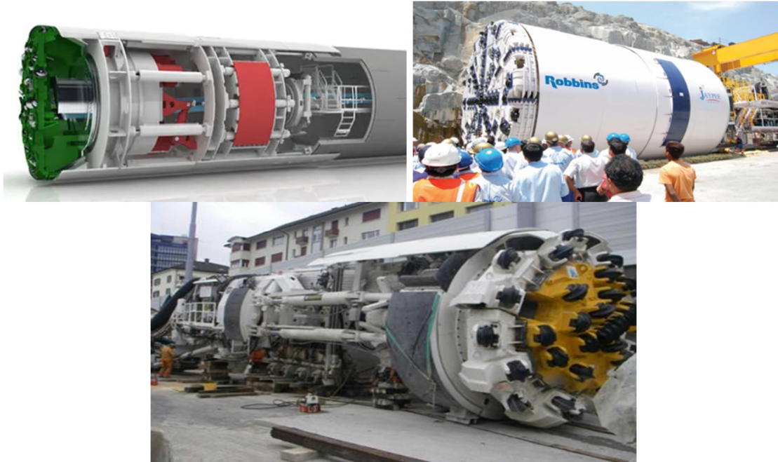
Figure 4-10 (Top) Open Double Shield for Rock; (Bottom) Open-Gripper TBM
