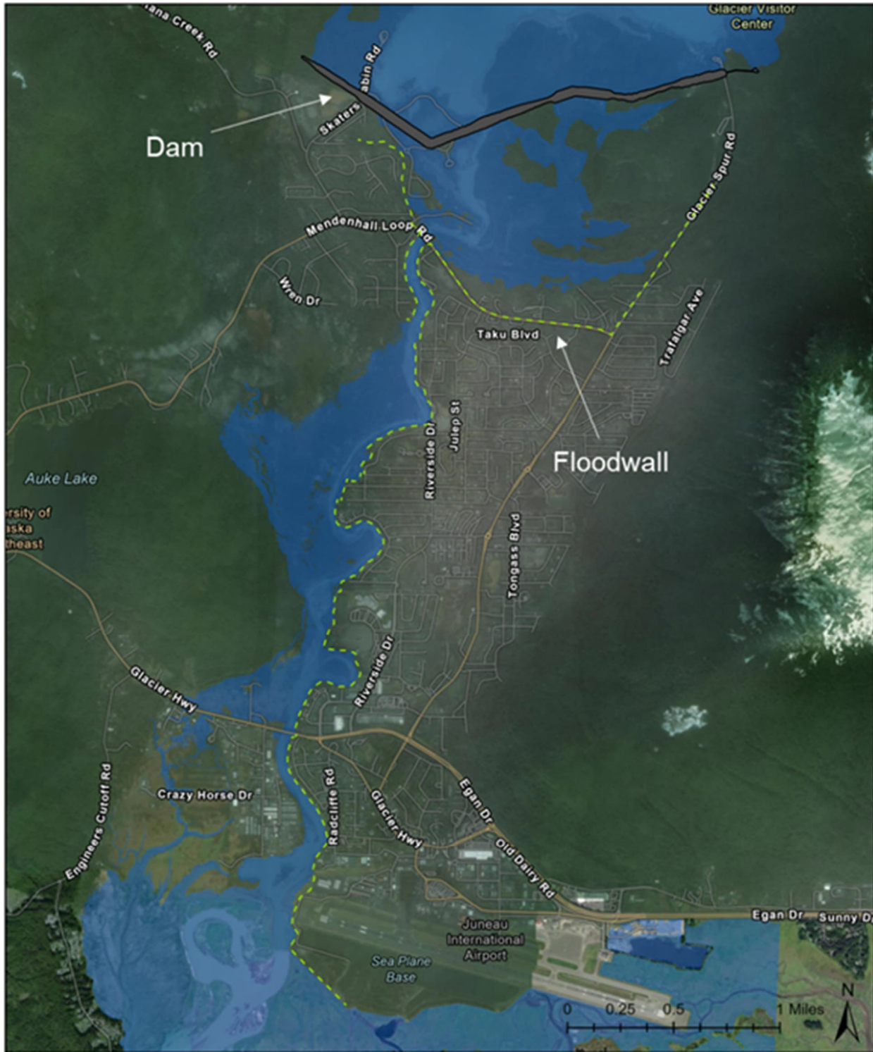
Figure 2-7 Floodwalls and Dam Shown with a Dam Release of 50,000 cfs
