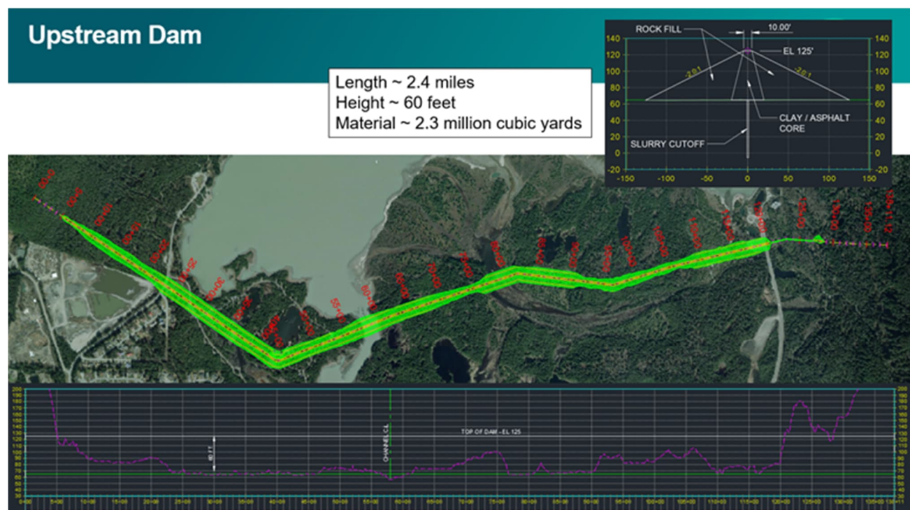
Figure 2-5 Dam Alternative Plan and Profile (Approximate)
