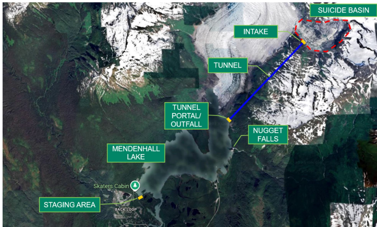
Figure 4-1 Lake Tap Tunnel Alternative Overview
