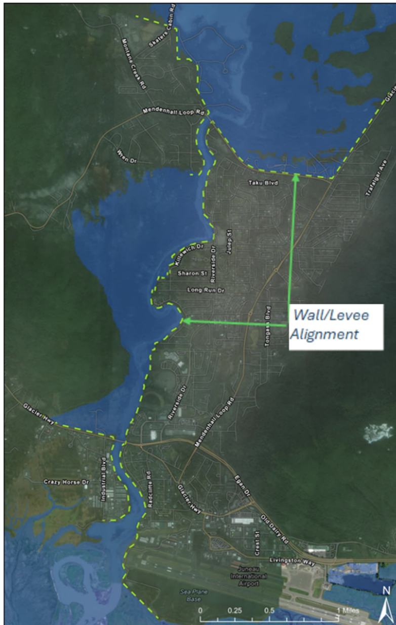
Figure 4-34 Floodwall Alternative: Inundation Extent and Alignment
